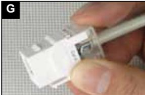
**G** Install dust caps by snapping into place as shown. Note: The cable jacket should remain outside the dust caps as shown.
